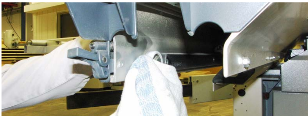
Fig. 7-6 Cleaning of the sub-rollers of the sliding table
