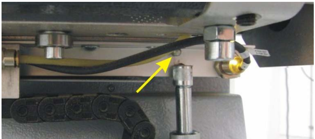
Fig. 7-14 Lubricating nipple, spindle drive F45
