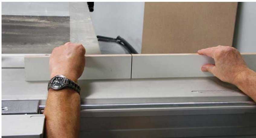
Fig. 5-45 Checking the 0° -setting
