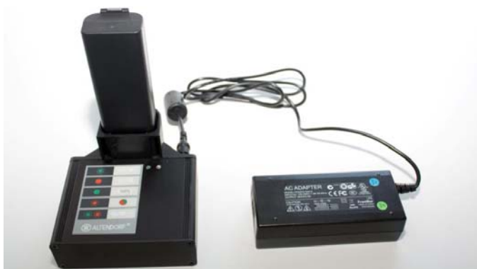
Fig. 6-81 Changing the rechargeable battery for WGA DIGIT LD
